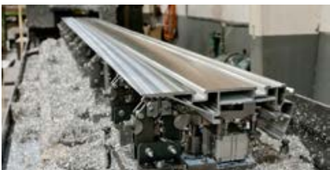
Milling of sliding table surface
